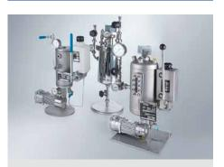
Depending on the design, application and mode of operation, mechanical seals and magnetic couplings need supply units for flushing, cooling, pressurization and leakage compensation.
